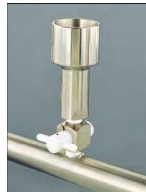
Standard branch accepts a #8 or #8b stopper, 2-way valve.
