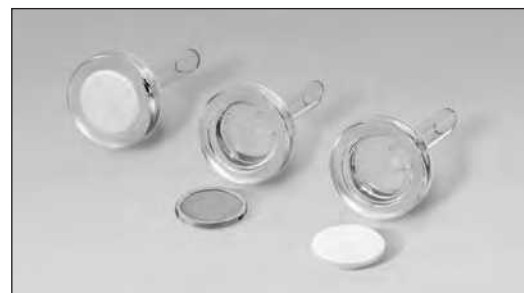
Glass frit, stainless steel support, PTFE support
